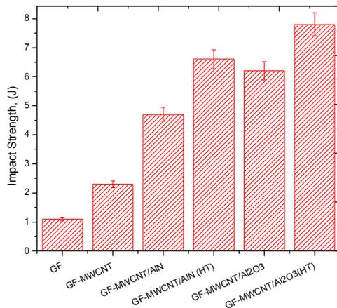
**Figure 4. Impact Strength of Glass-Epoxy based composites**
