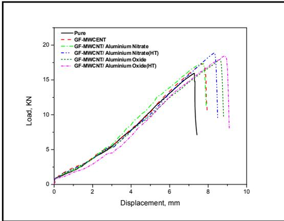
Figure 2. Typical Load Vs Displacement curves obtained from tensile tests of Glass-Epoxy based composites
