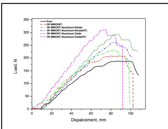
Figure 3. Typical Load Vs Displacement curves obtained from Flexural tests of Glass-Epoxy based composites
